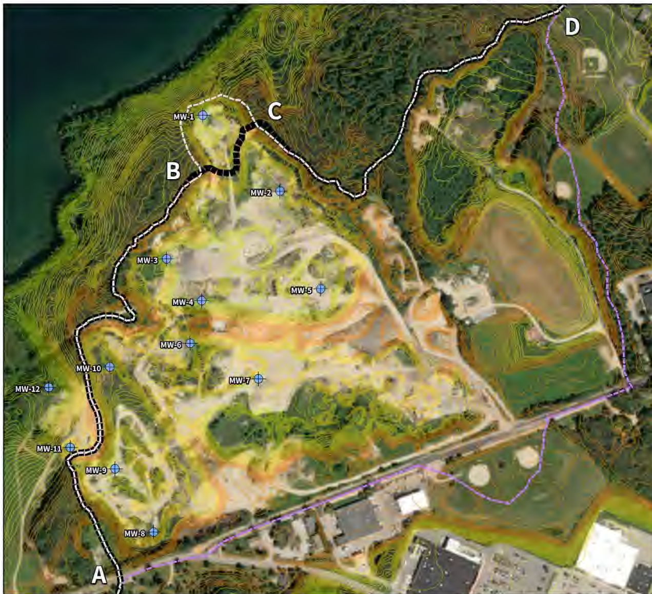
Figure 1. Tentative 2022 revision #2 (white dashed line) of the 2021 revised watershed boundary (black dashed line) compared to the pre-2021 original watershed boundary (purple dashed line) for Lake Auburn. Letters A, B, C, and D indicate start and end points of segments described in the text.
