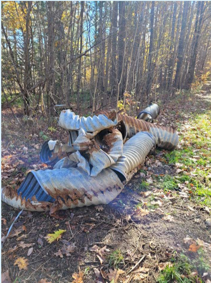
An older metal culvert that has rusted.
